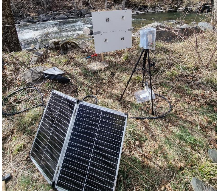
Figure 1: Abundance/Biomass monitoring system. In the picture are visible the target (white panel) with Aruco codes for image geometry wrapping, the camera system and the solar energy battery system
